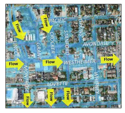
Figure 6 - Problem Area 3 Simulated Flooding
