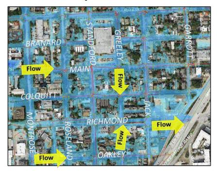
Figure 7 - Problem Area 4 Simulated Flooding
