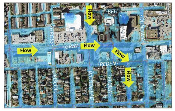
Figure 4 - Problem Area 1 Simulated Flooding
