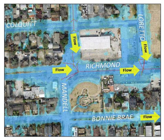
Figure 8 - Problem Area 5 Simulated Flooding
