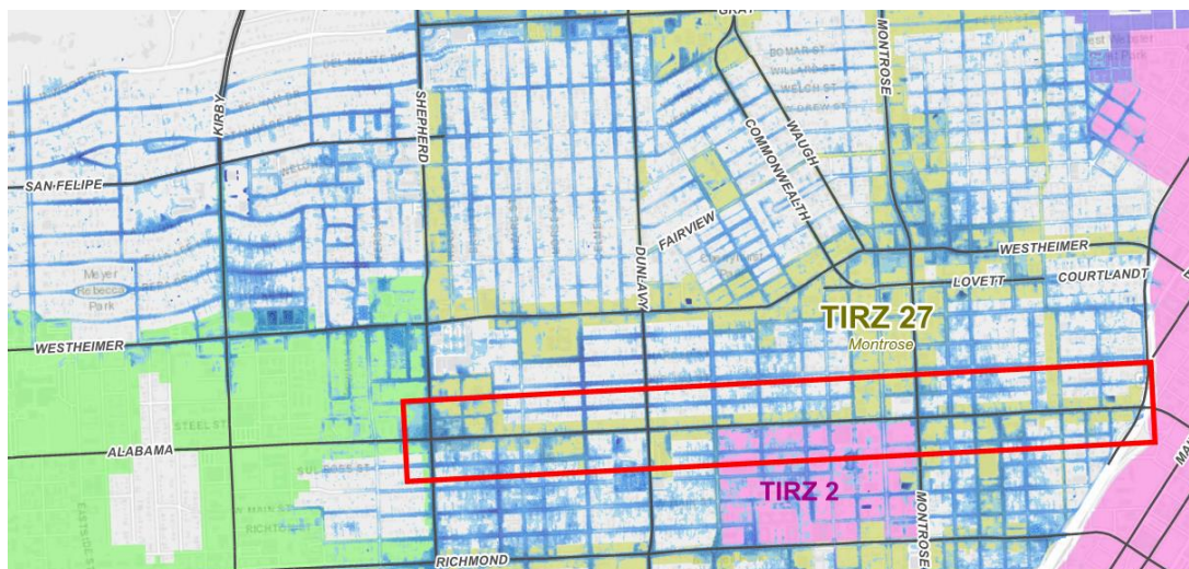
Figure 2: 100-yr Ponding on West Alabama within proposed project limits
