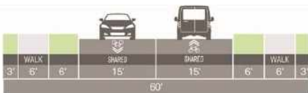
30-FT Curb to Curb Width Section
