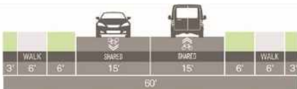
30-FT Curb to Curb Width Section
