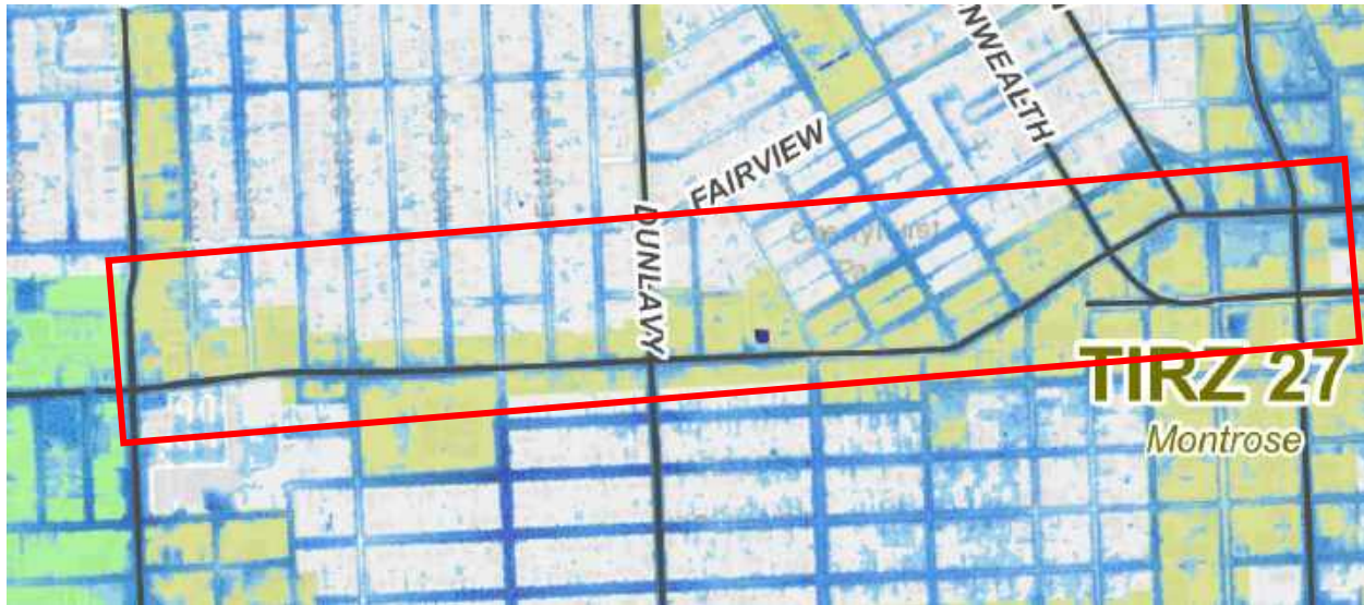
Figure 2: Existing 100-yr ponding on Westheimer Road within proposed project limits
